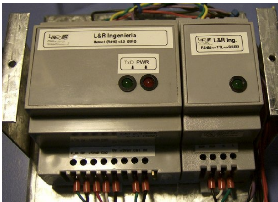
Figure 1 View of the METEO module with associated RS-485 interface
